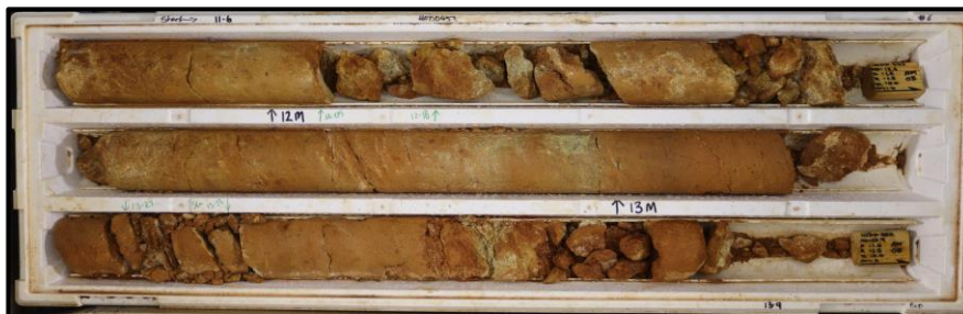
Type S1 (Below Water Table) and T1 (Above Water Table) – Upper Alluvium
