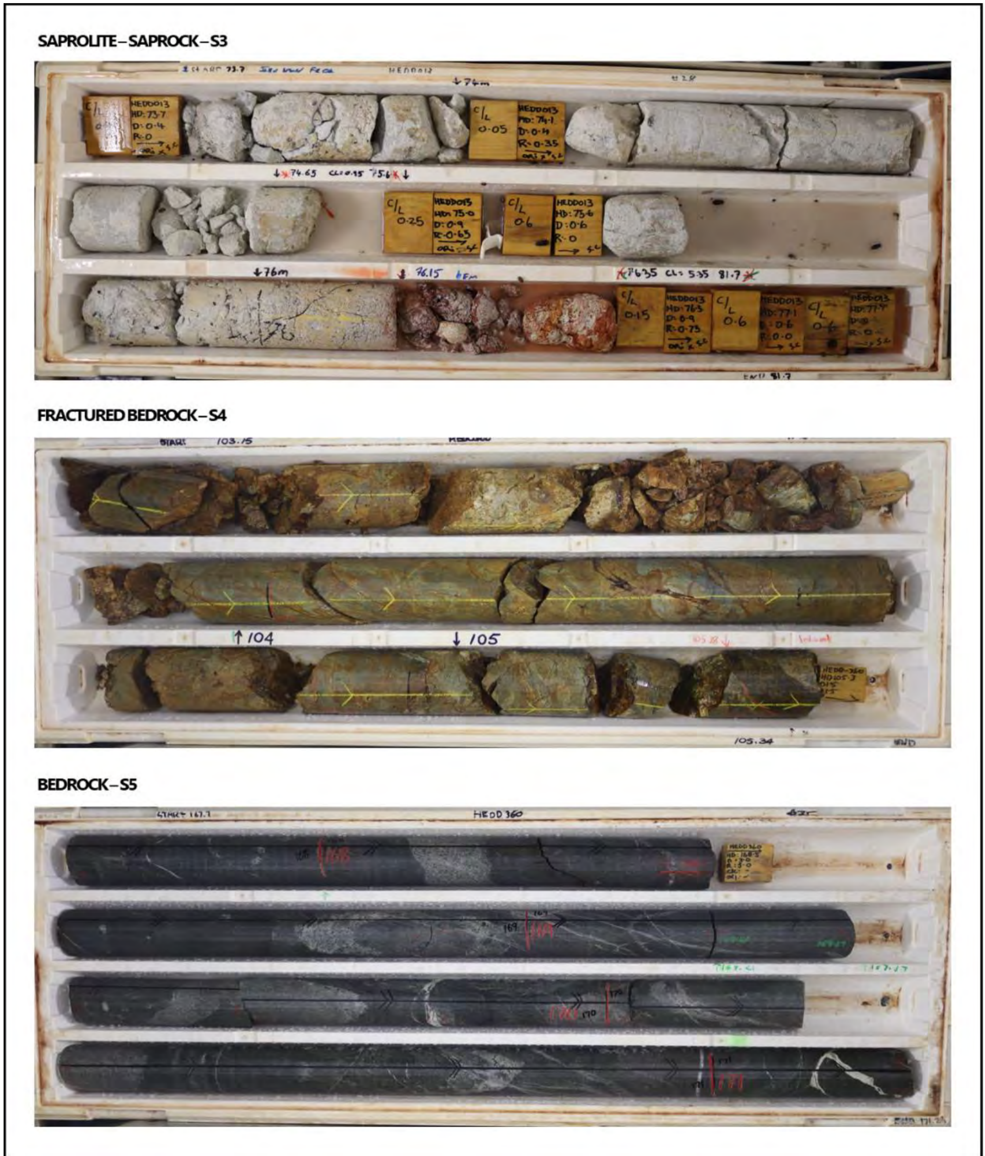
Plate 6-2: Diamond Drill Core Examples of the Saprolite – Saprock (S3), Fractured Bedrock (S4) and Bedrock (S5) Geological Domains
