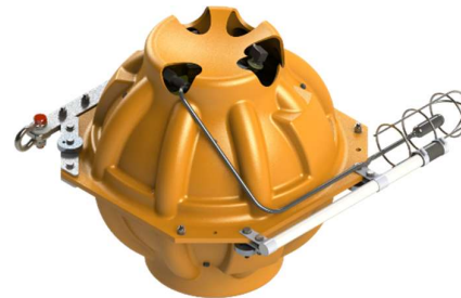
Figure 12. Acoustic recording equipment used in this study: (Left) JASCO’s ALTO lander ready for deployment, containing AMAR, hydrophones, floats, and acoustic release, and (right) JASCO’s AMAR Generation 4 Ultra Deep (AMAR G4 UD) acoustic recorder with hydrophone.
