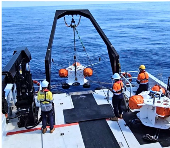
Figure 12. Acoustic recording equipment used in this study: (Left) JASCO’s ALTO lander ready for deployment, containing AMAR, hydrophones, floats, and acoustic release, and (right) JASCO’s AMAR Generation 4 Ultra Deep (AMAR G4 UD) acoustic recorder with hydrophone.
