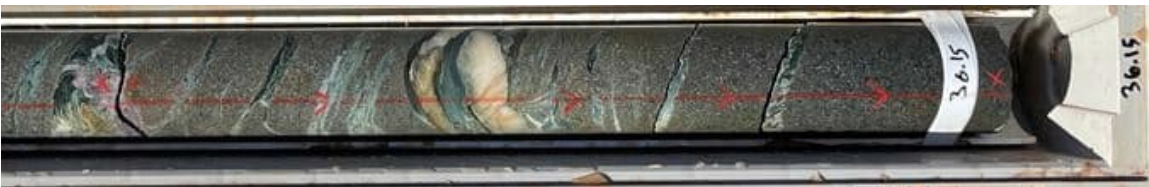
Photo 4. W1/SP0-BH24 – example of potential fibrous seams, 1 mm to 50 mm thick encountered between 27.9 m and 49.05 m
