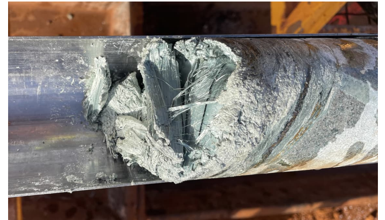
Photo 6. W1/SP0-BH19 – potential fibrous seam between defect (61.7 m to 61.9 m)
