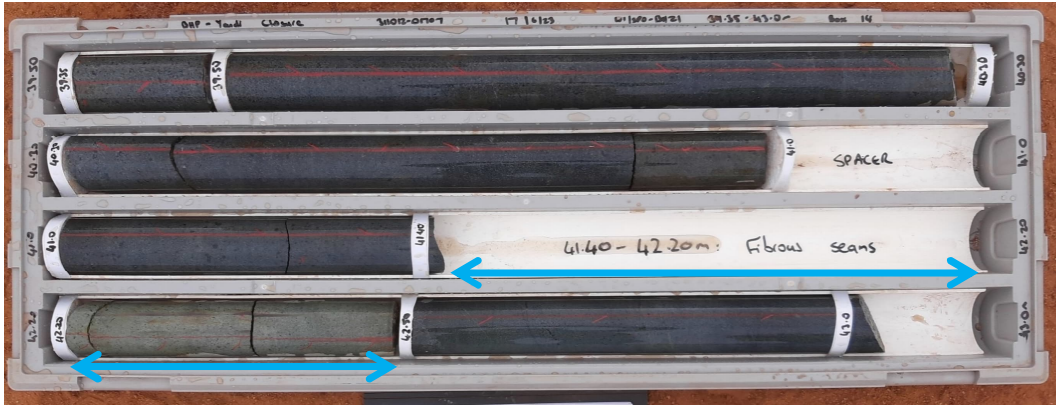
Photo 1. W1/SP0-BH21 showing ~1 m layer of medium-grained grey dolerite within fine- to medium-grained dark grey dolerite (section of medium-grained grey dolerite core removed from 41.4m to 42.2m where potential fibrous seams noted – see Photo 2)
