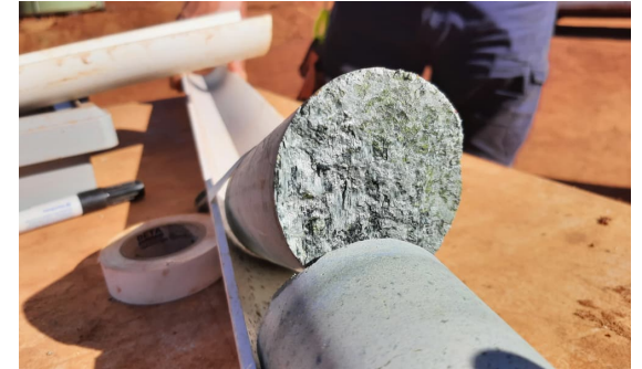
Photo 5. W1/SP0-BH26 – 2 mm thick potential fibrous seam between joint at 29.9 m and 30.15 m
