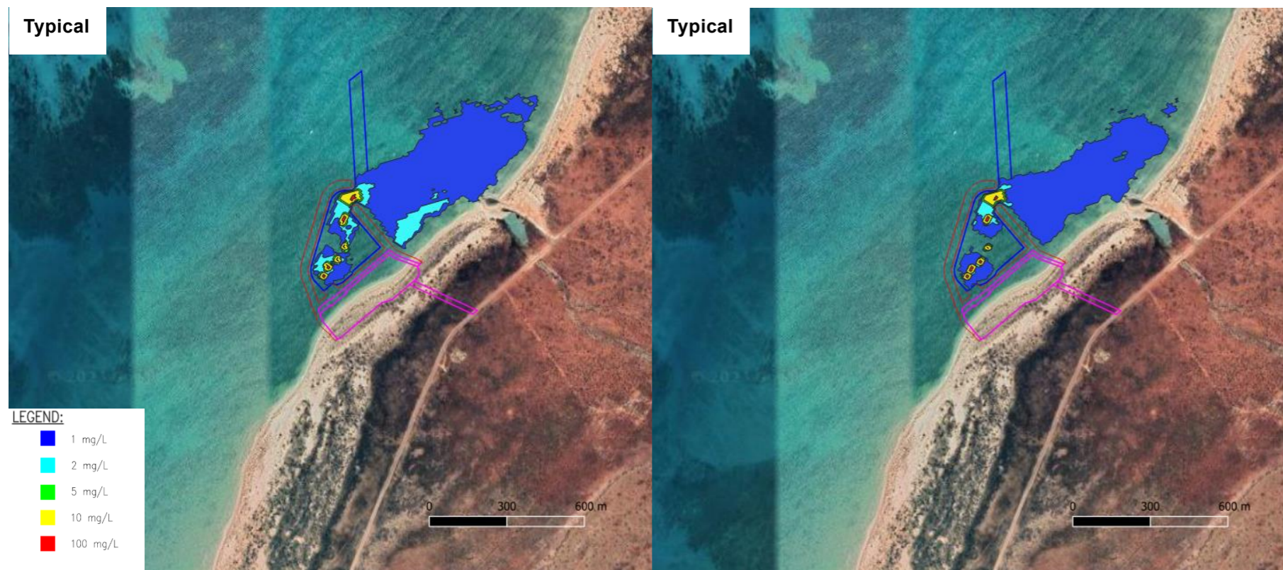
Figure 5.5 95% Exceedance Near Field Plots for Winter (Run 1, left), & Summer (Run 5, right) for Comparison
