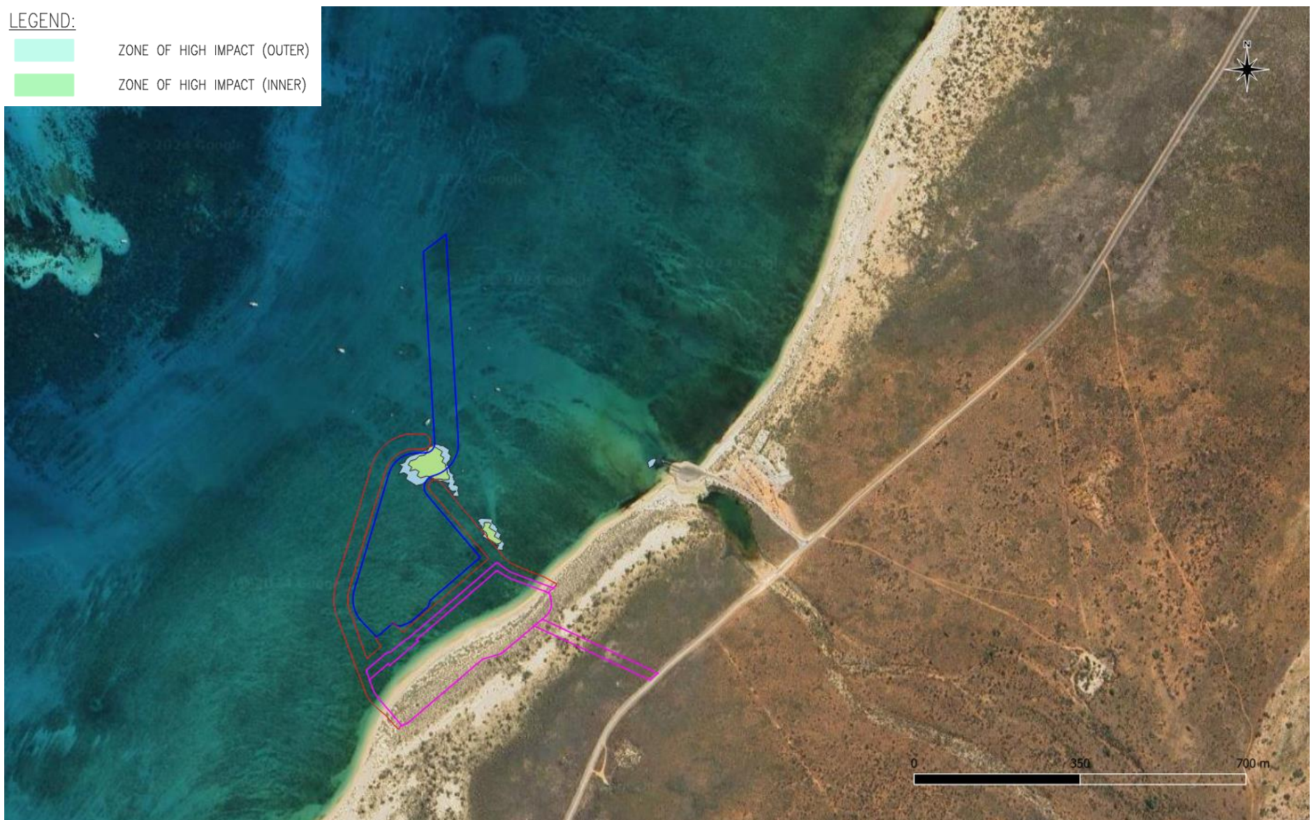
Figure 4.2 Run011 Sedimentation 95% Exceedance Plot
