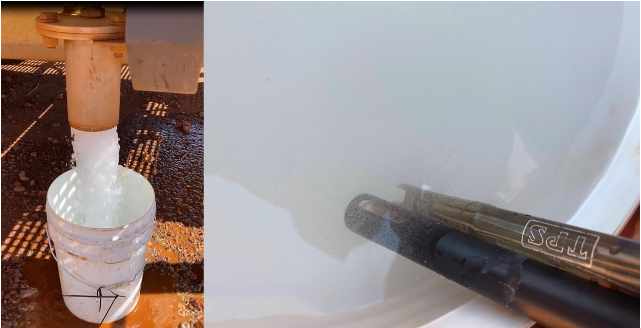
Figure 5-4: Photo showing sampling of groundwater from production bore HGE0148P (left) and bubbles (likely CO 2 ) forming shortly after sampling (right).
