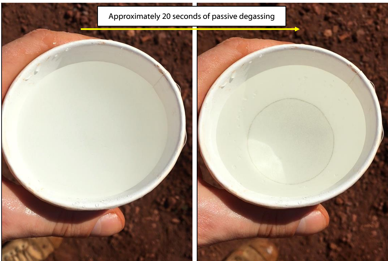
Figure 5-5: Groundwater immediately after sampling (left panel) has a cloudy appearance [bottom of the cup is not visible] due to the presence of abundant gas bubbles (likely CO 2 – as indicated by gas monitoring equipment – see Section 5-24). Groundwater sample after exposure to ambient surface pressure and temperatures for approximately 20 seconds (right panel) has degassed significantly (very few CO 2 bubbles) resulting in a transparent appearance.
