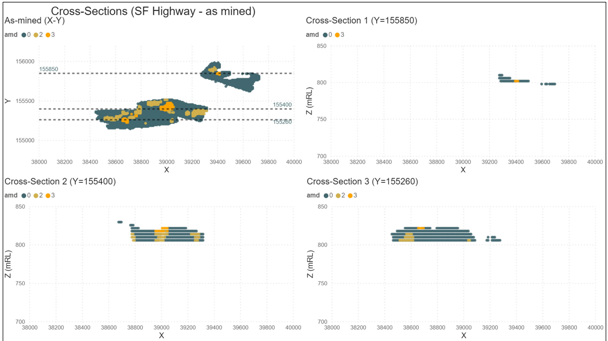
Figure 3-96 Spatial variability (2D X-Y view and cross sections) of as-mined AMD material predicted by SF Highway deposit mining model (including all waste rock, low grade ore and ore blocks)
