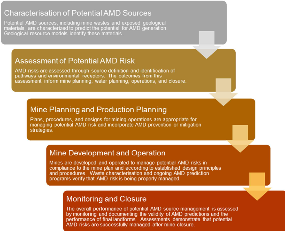
Figure 1-1 AMD Management process flow (BHP, 2018a)
