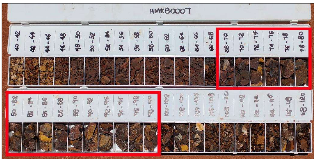
Figure 16: HMKB0007M: Broken Ground
