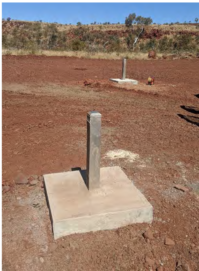
Plate 1: Typical headworks completion of monitoring bores (HMN0016M deep and HMN0015M shallow)
