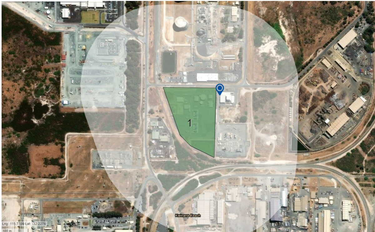
Figure 9-1 Project area and defined buffer zone with radius of 300 m from the premises boundary.
