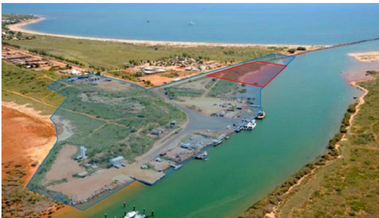
Figure 1 Existing Beadon Creek Maritime Facility (shaded blue), including existing OMSB land-backed wharf facility (OMSB Project Stage 1) footprint (shaded red) (Source: BMT Oceanica 2015)
